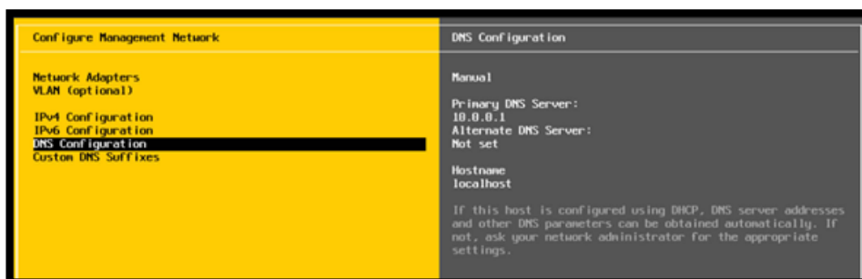
Figure 4- 4: Configuration du serveur DNS
