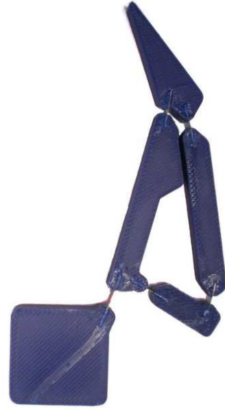
(a) Prototype with joints made of nitinol (Boudreault and Gosselin, 2006).
