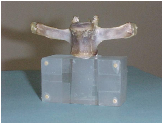
FIGURE 5: Picture of the realised calibration model. The dried sheep vertebra (anterior view) fixed to a radiographically transparent Perspex block measuring 72 mm by 40 mm by 34 mm with eight 3 mm diameter metallic markers inserted.
