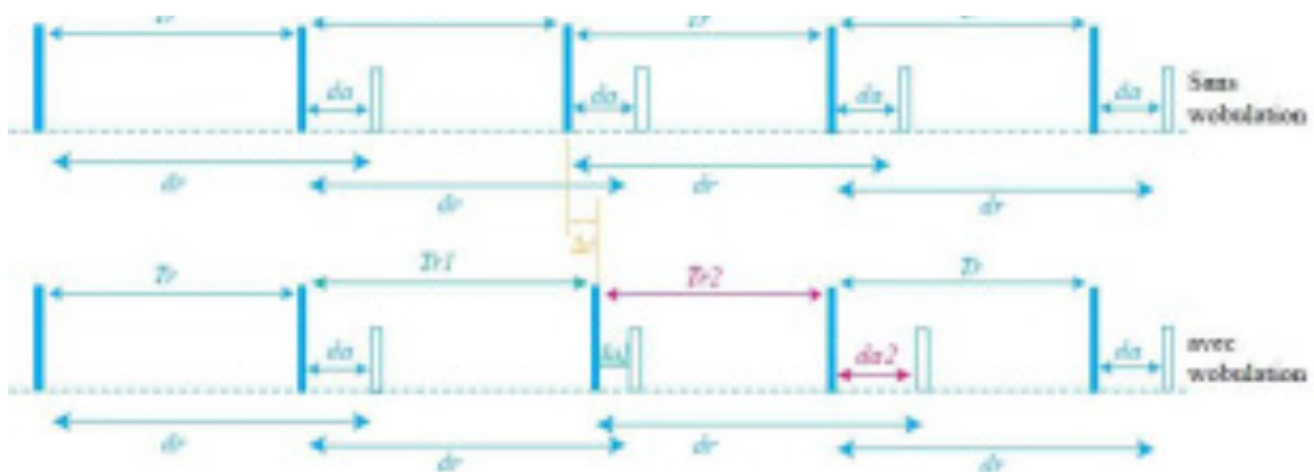
Figure 48:principe de wobulation
