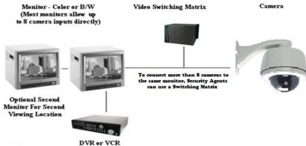
Fig. II. v: CCTV Running
