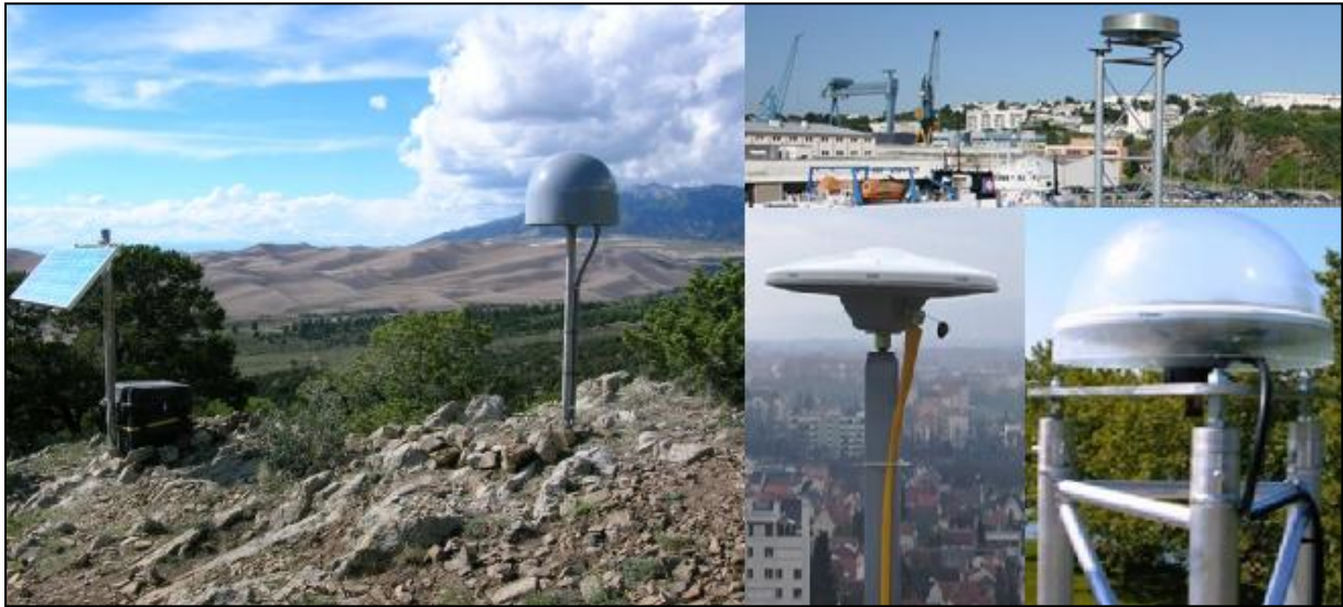
Figure 1 : Station Permanente GNSS
